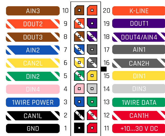
Figure 2 FMM640 pinout
